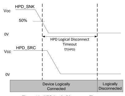
Figure 12. HPD Logic Disconnect Timeout
