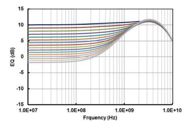
Figure 26. Adaptive EQ Gain Curve
