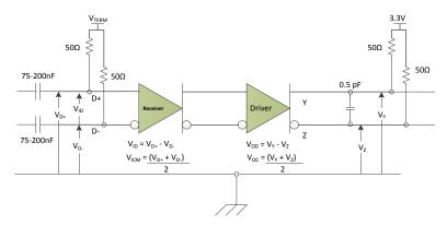
Figure 1. TMDS Main Link Test Circuit
