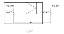
Figure 10. HPD Test Circuit
