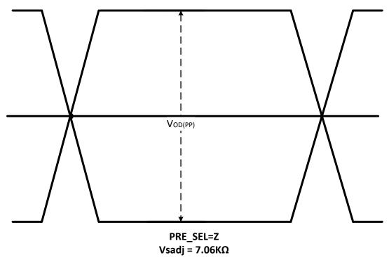
Figure 5. Output Differential Waveform 0 dB De-Emphasis
