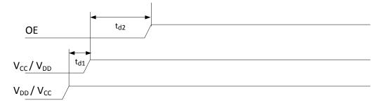
Figure 22. Power-Up Timing for SNx5DP159
