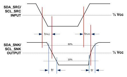
Figure 15. DDC Propagation Delay - Source to Sink
