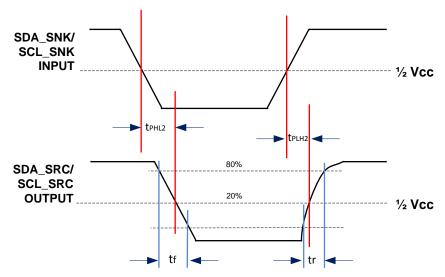
Figure 16. DDC Propagation Delay - Sink to Source
