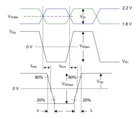
Figure 2. Input and Output Timing Measurements
