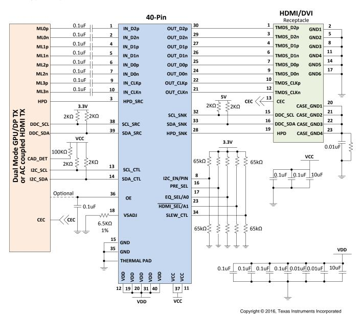
Figure 33. Implementation for Motherboard 1 Schematic
