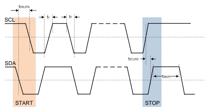
Figure 13. Start and Stop Condition Timing
