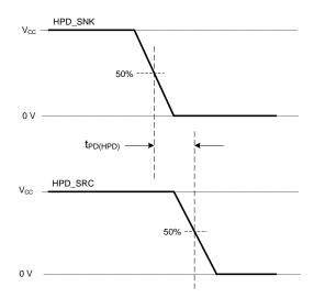
Figure 11. HPD Timing Diagram Number 1
