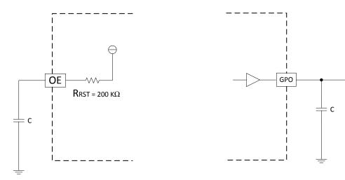
Figure 20. External Capacitor Controlled OE
