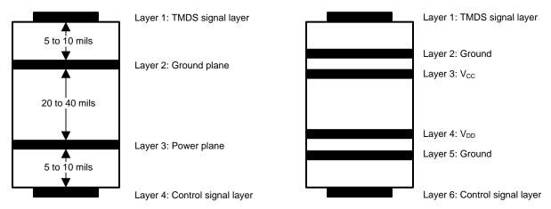
Figure 35. Recommended 4- or 6-Layer Stack for a Receiver PCB Design
