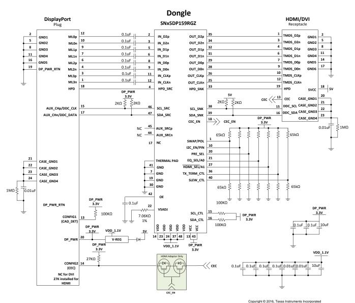
Figure 32. SNx5DP159 in Dongle Application
