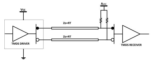
Figure 27. TMDS Driver and Termination Circuit
