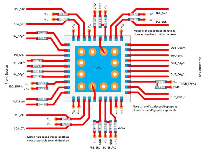
Figure 36. Layout Example for the DP159RSB
