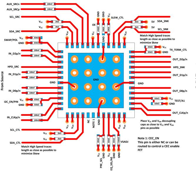
Figure 37. Layout Example for the DP159RGZ
