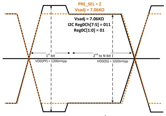
Figure 29. Pre-Emphasis Using I<sup>2</sup>C Method
