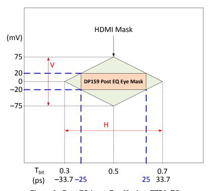
Figure 8. Post EQ Input Eye Mask at TTP2\_EQ
