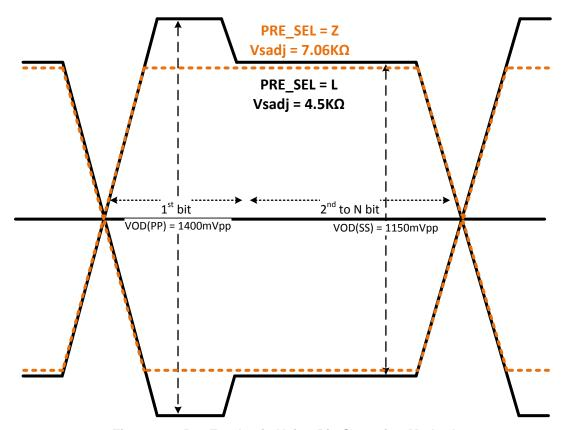
Figure 28. Pre-Emphasis Using Pin Strapping Method
