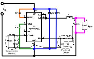
Figure 2. Current Path Diagram
