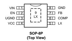
The Pin 5 must be connected to the Exposed Pad
