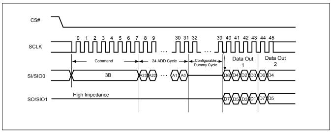
Figure 29. Dual Read Mode Sequence (SPI Mode only)
