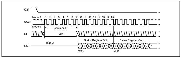
Figure 19. Read Status Register (RDSR) Sequence (QPI Mode)
