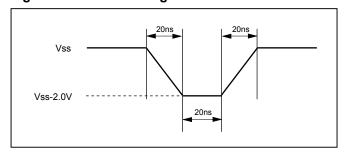
Figure 73. Maximum Positive Overshoot Waveform
