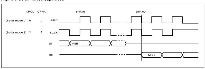
Figure 1. Serial Modes Supported
