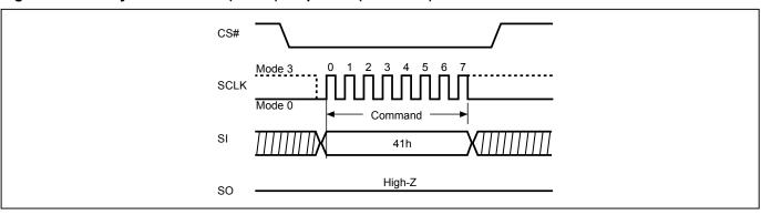
Figure 11. Factory Mode Enable (FMEN) Sequence (QPI Mode)
