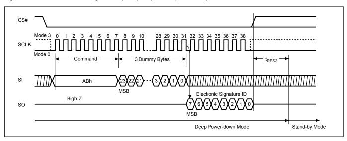
Figure 13. Read Electronic Signature (RES) Sequence (SPI Mode)
