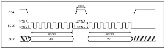
Figure 70. Reset Sequence (QPI mode)
