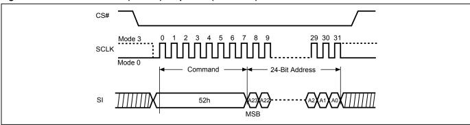
Figure 41. Block Erase 32KB (BE32K) Sequence (QPI Mode)
