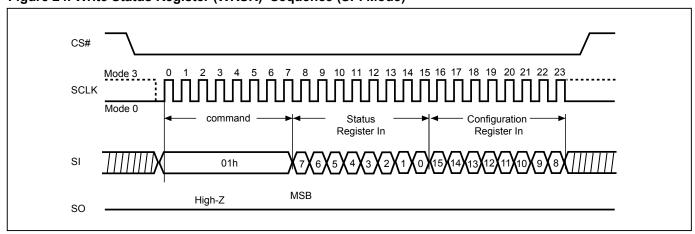
Figure 24. Write Status Register (WRSR) Sequence (SPI Mode)
