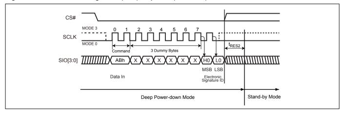
Figure 15. Release from Deep Power-down (RDP) Sequence (SPI Mode)
