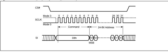
Figure 43. Block Erase (BE) Sequence (QPI Mode)
