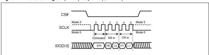
Figure 25. Write Status Register (WRSR) Sequence (QPI Mode)
