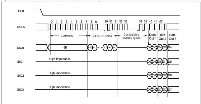
Figure 31. Quad Read Mode Sequence (SPI Mode only)
