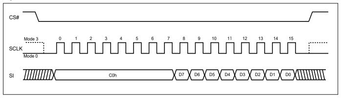
Figure 35. Burst Read - QPI Mode
