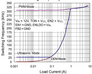
VOUT1 Switching Frequency vs. Load Current
