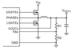
Figure 6. Setting VOUTx with a Resistor-Divider
