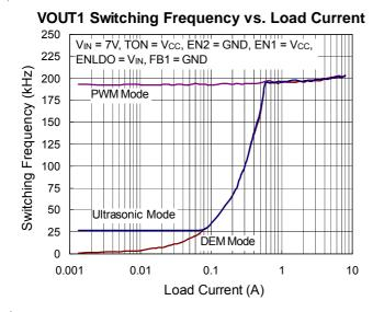
**VOUT1 Switching Frequency vs. Load Current**
