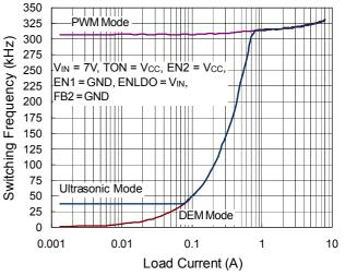
VOUT2 Switching Frequency vs. Load Current
