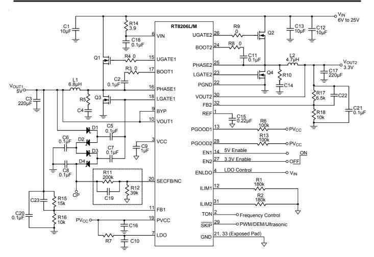
Figure 2. Adjustable Voltage Regulator
