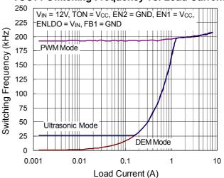
VOUT2 Switching Frequency vs. Load Current
