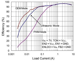
VOUT2 Efficiency vs. Load Current
