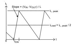
Figure 3. Boundary Condition of CCM/DEM
