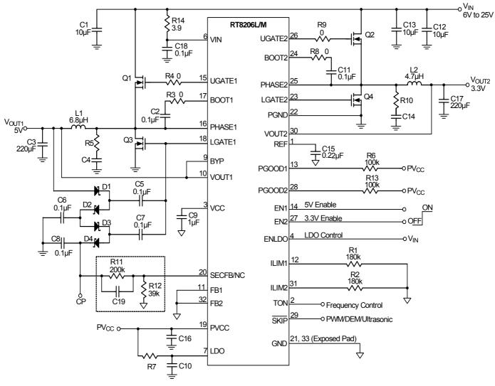
Figure 1. Fixed Voltage Regulator
