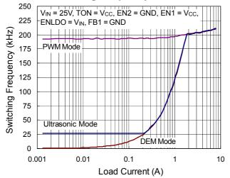
VOUT2 Switching Frequency vs. Load Current
