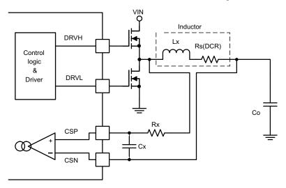
Figure 48. Inductor DCR Current Sensing
