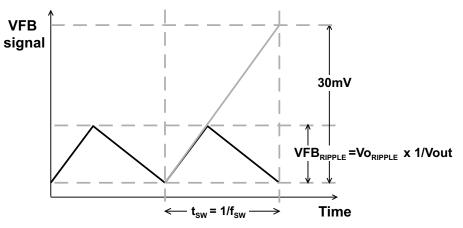
Figure 46. Required voltage feedback ramp signal
