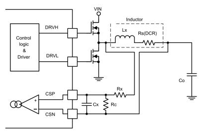
Figure 49. Inductor DCR Current Sensing With Voltage Divider
