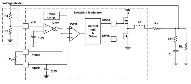
Figure 45. Simplified D-CAP Mode Functional Blocks
