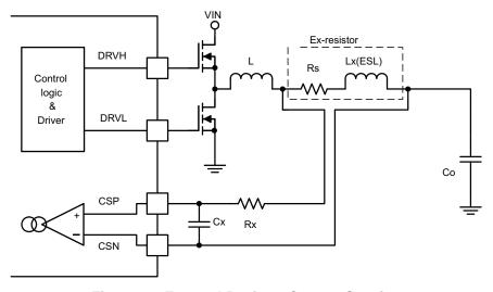
Figure 47. External Resistor Current Sensing
