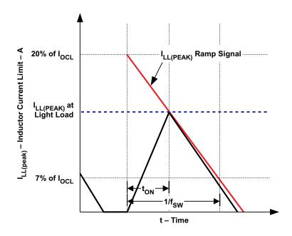
Figure 43. Inductor Current Limit at Pulse Skipping
