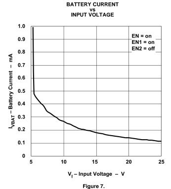
NO LOAD BATTERY CURRENT vs INPUT VOLTAGE
