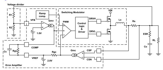
Figure 44. Simplified Current Mode Functional Blocks
