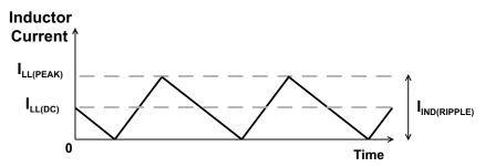
Figure 42. Boundary Between Pulse Skipping and CCM
