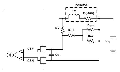
Figure 50. Inductor DCR Current Sensing With Temperature Compensate
