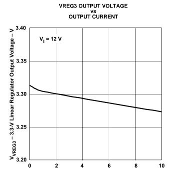
I<sub>REG3</sub> – 3-V Linear Regulator Output Current – mA Figure 9.
