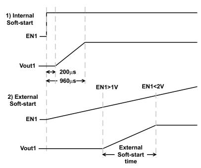
Figure 40. Enable and Soft-start Timing
