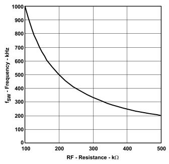
Figure 41. Switching Frequency vs RF
