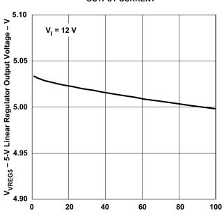
I<sub>REG5</sub> – 5-V Linear Regulator Output Current – mA
