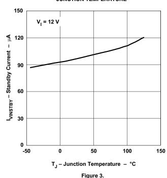
INPUT VOLTAGE SHUTDOWN CURRENT vs JUNCTION TEMPERATURE
