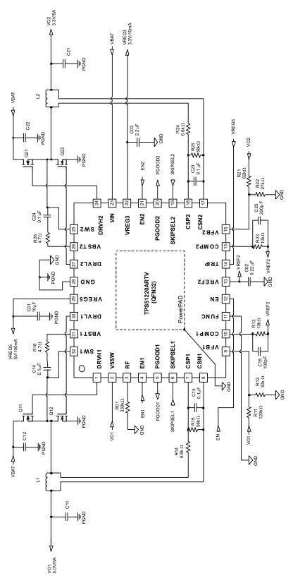
Figure 57. Current Mode, DCR Sensing, 5.0-V/5-A, 3.3-V/5-A, 300-kHz
